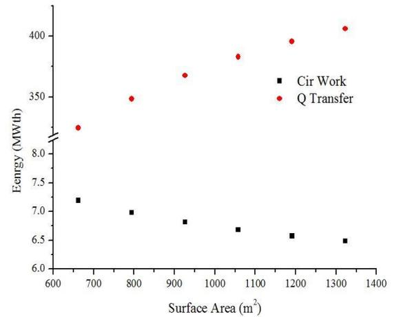
Fig.4. Circulator work and Q transfer in variable heat structure areas for He.
