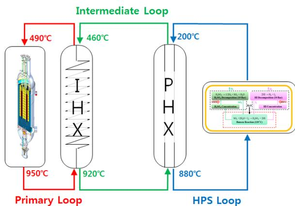
Fig. 1. Schematic diagram of nuclear hydrogen production system.
