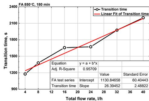
Fig. 3. Time to transition and linear fitting curve of FA 850°C test series
