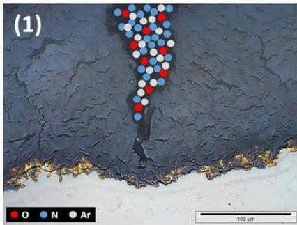
(1) At initial phase, mixed atmosphere would be located at crack tips maintaining equivalent concentration with purge gas
