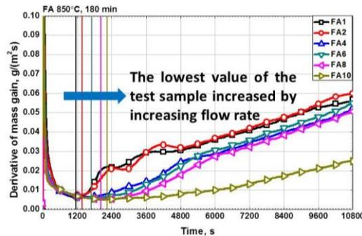
Fig. 2. Derivatives of FA 850°C test series
