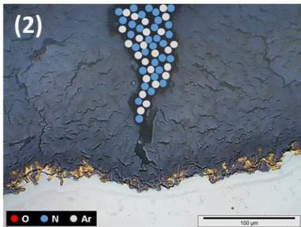
(2) Oxygen would react firstly with zirconium metal because of its high reactivity.
