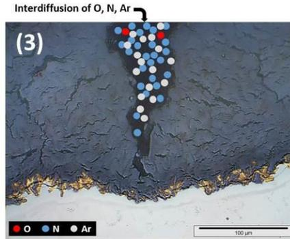
(3) Oxygen in flowing gas diffuses into the crack tips, oxide scale and metallic part.
