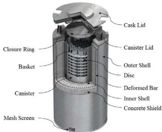
Fig. 1. Configuration of concrete storage cask
