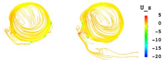
Fig. 3. Comparison of flow streamlines around containment between orientations A (left) and B (right).
