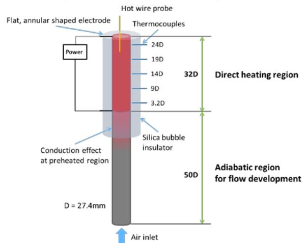
Fig. 1. Schematic diagram of the test section of Shehata's experiment
