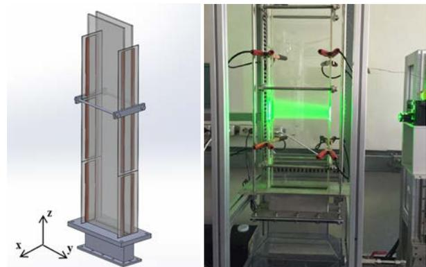
Fig. 5. Design of test section with FTO coated heat-resistant glass (left) and picture of the test section of the facility (right)
