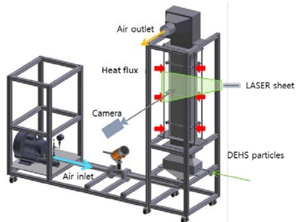
Fig. 4. Design of the flow visualization test facility
