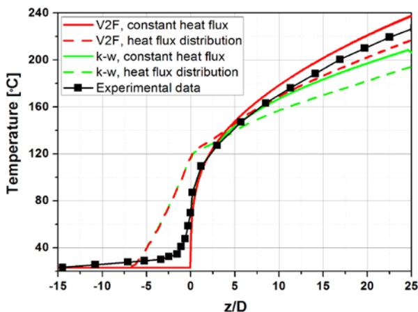
Fig. 2. Wall temperature distribution along the axial direction from the entry of the heated tube for the two boundary conditions with two turbulence model
