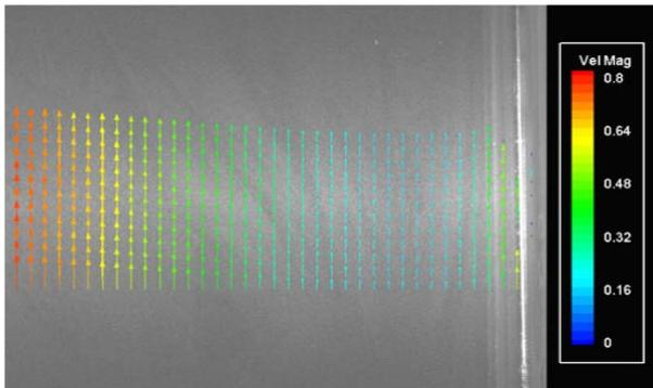
Fig. 6. Mean velocity field obtained with PIV method at the mid-plane in the depth direction
