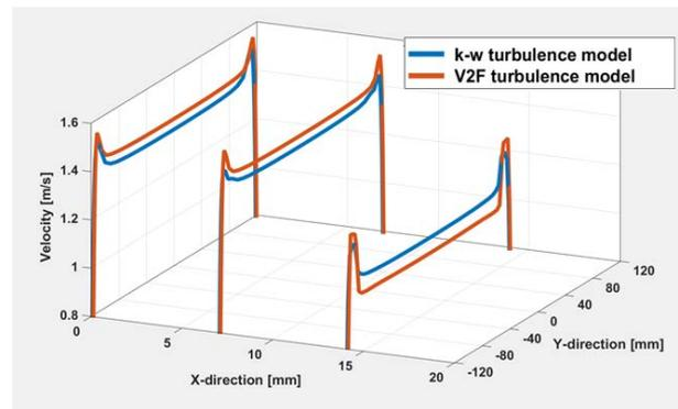
Fig. 3. Local vertical velocity profiles at the mid-plane ( $x = 0$  mm),  $x = 7$  mm and  $x = 14$  mm of certain height in the heated rectangular riser duct
