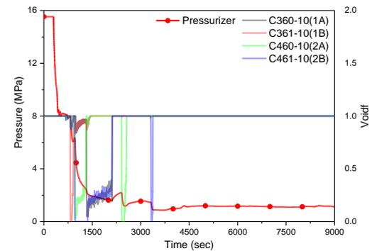
Fig. 6. The pressurizer pressure and liquid fraction of the horizontal intermediate legs for the MARS
