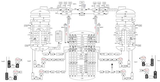
Fig. 2. MARS-KS nodalization for the ATLAS LTC-CL-04R
