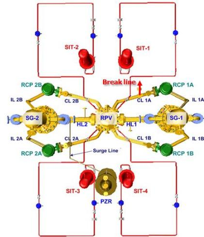
Fig. 1. Schematic diagram of the ATLAS and break position
