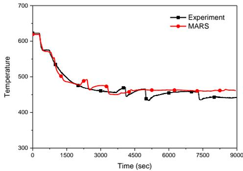
Fig. 7 The cladding temperature
