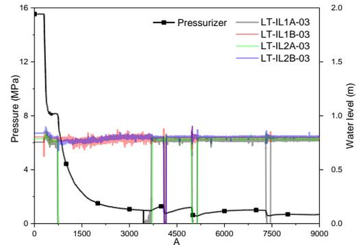
Fig. 5. The pressurizer pressure and water level of the horizontal intermediate legs for the experiment
