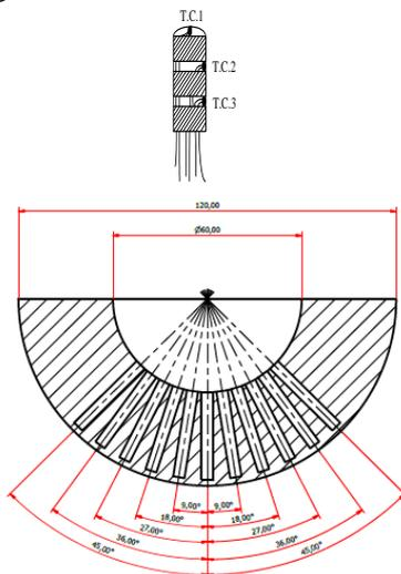
Fig.1 Schematics of a heat flux sensor (up) and channels to hold heat flux sensors (bottom).
