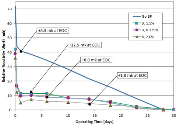
Fig. 2. Reactivity Swing vs. Boron Concentration in the HANARO Core Consisting of All Standard Fuel Rods
