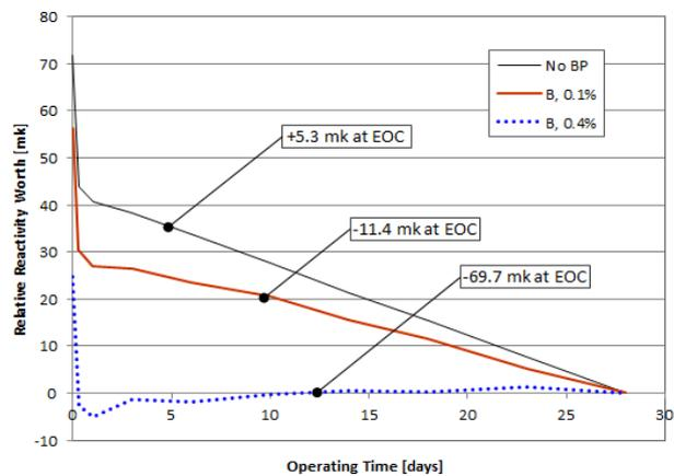
Fig. 1. Reactivity Swing vs. Boron Concentration in the HANARO Core
