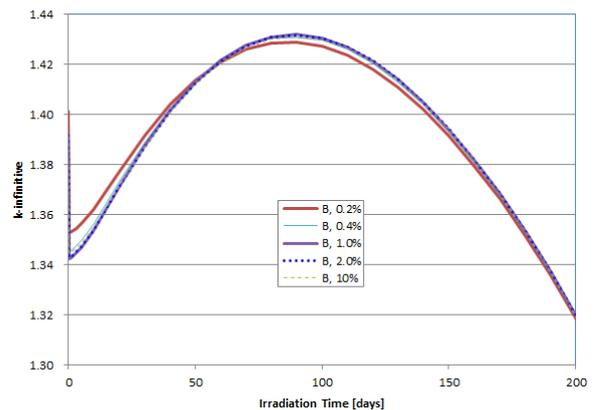
Fig. 5. Reactivity Rundown Curves for Each Boron Concentration
