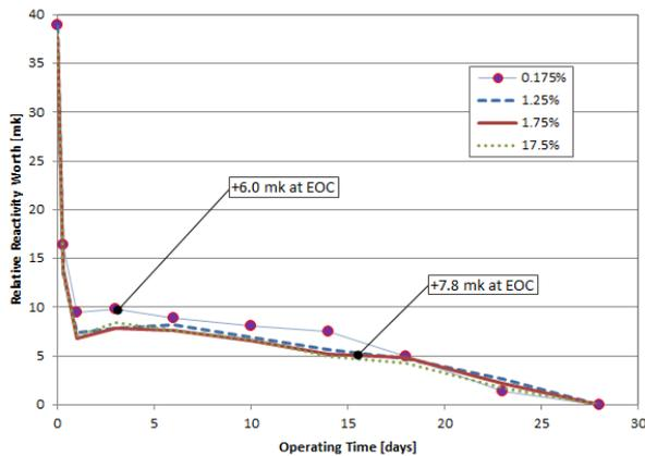
Fig. 6. Comparison of the Reactivity Swings for Several Boron Concentration Cases.
