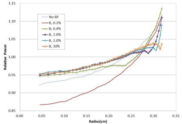
Fig. 4. Relative Power Distribution with the Fuel Rod for Each Boron Concentration
