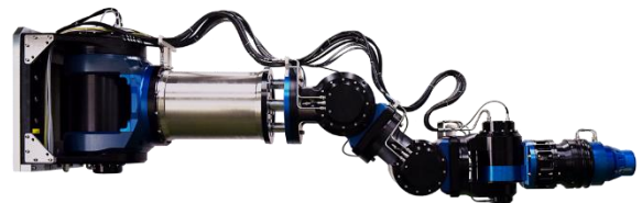
Fig. 3. The picture of the developed hydraulic manipulator using the developed hydraulic actuator modules for dismantling the reactor pressure vessel of nuclear power plants
