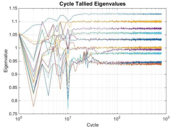
Fig. 3. Eigenvalues tallied at every cycle as the ratio of the total absolute weight values to the number of histories per cycle.
