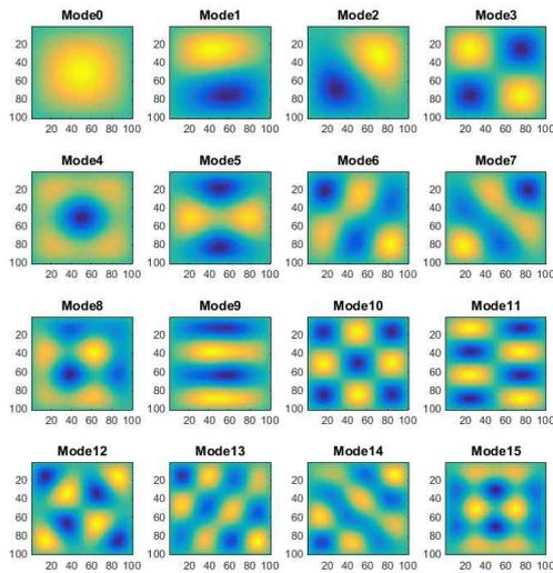
Fig. 5. The fission source distributions of the first 16 eigenmodes.
