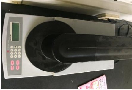
Fig.4 Four probe resistivity measurement system (AIT, CMR-SR 1000N)
