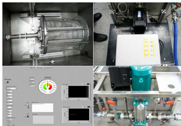
Fig. 5. Build a stirring device. (stirring vessel, motor controller, circulation pump and control program. Clockwise , from top left)
