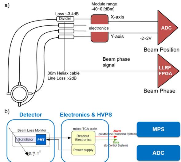
Fig. 2. Schematics of data acquisition of beam signals from the detectors for a) beam position monitor and b) beam loss monitor.
