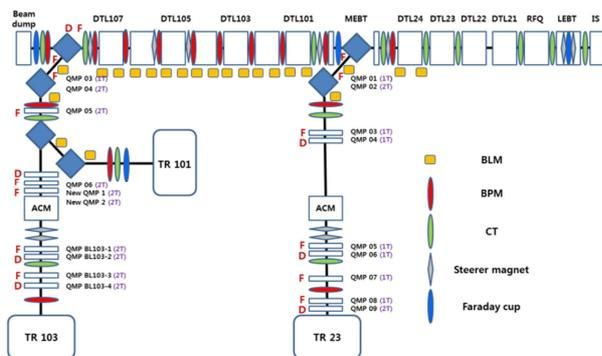
Fig. 1. Layout of beam diagnostics in KOMAC linac and beam lines
