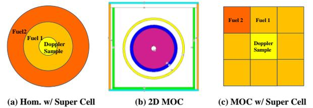
Fig. 6. MC<sup>2</sup>-3 Doppler sample models
