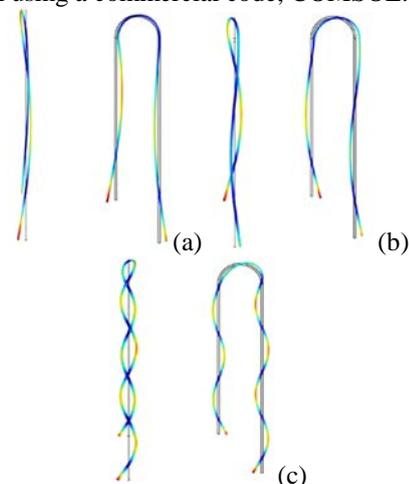
Fig. 3. Mode Shapes Computed: (a) Mode 1, 26 Hz, (b) Mode 2, 43 Hz, (c) Mode 3, 301 Hz.
