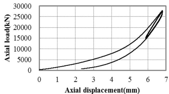
Fig. 3. Axial Characteristic Curve
