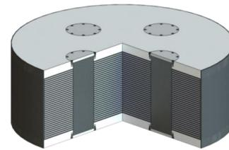
Fig. 2. Concept of Multi-lead Rubber Bearing (MLRB)
