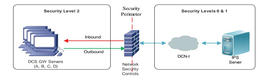
Establishing a Security perimeter between the DCN-I Subnetwork and redundant safety channels gateway servers to implement cybersecurtiy access controls to control and manage the inbound data traffic (On-demand traffic).
