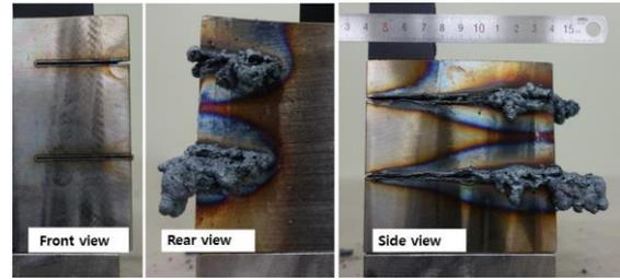
Fig. 2 Stainless steel after cutting (thickness: 100 mm, nozzle throat: 4mm, cutting speed: 45 mm/min and 50 mm/min)
