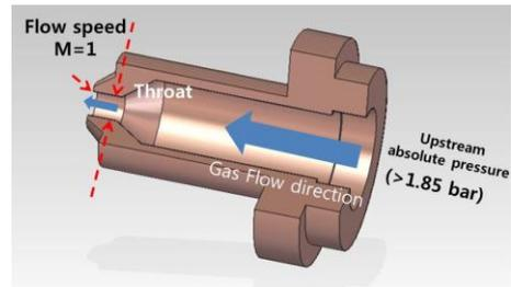
Fig. 1 Internal structure of converging nozzle.
