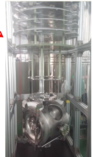
Vertical cavity test
