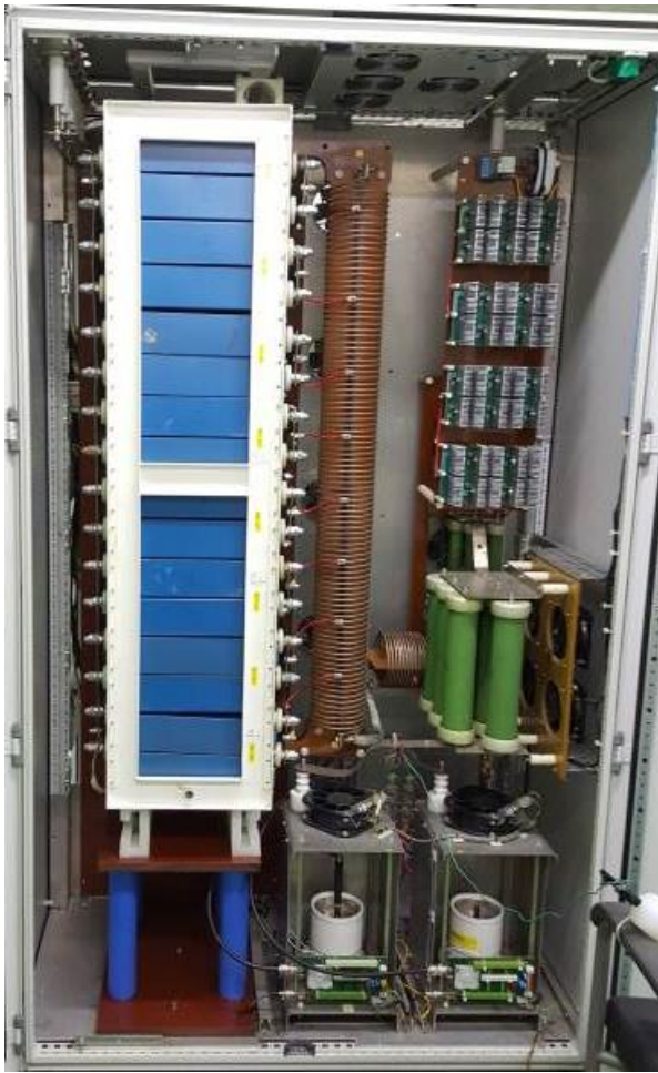
Fig. 3. Rusty modulator for 10 MeV accelerator
