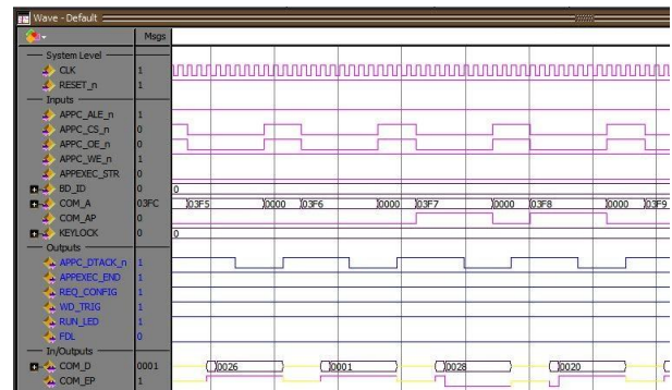
Fig. 3. The waveform of the pre-synthesis simulation results.
