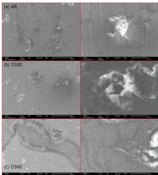
Fig. 3. Worn surface morphology after fretting wear tests.
