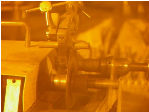
Fig. 1. Cutting of the irradiated cladding using the micro-cutting machine in a hot cell.
