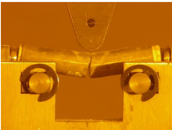
Fig.5. Fractured behavior of the irradiated cladding for the three-point bending test with alumina pellets in a hot cell.
