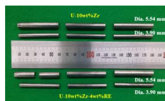
Fig. 5. Photography of final fuel slug after machining; U-10wt.%Zr (upper), U-10wt.%Zr-4wt.%RE (lower).
