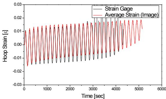
Fig. 4. Comparison of response measured by strain gage
