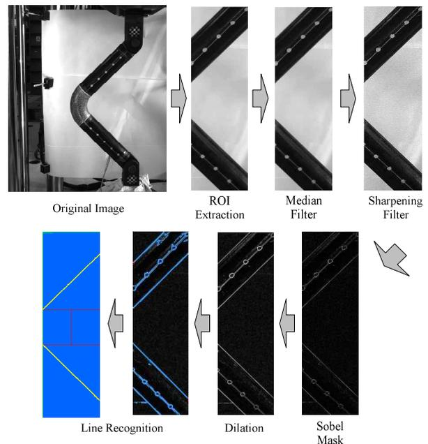
Fig. 2. Deformation angle measurement using image signal
