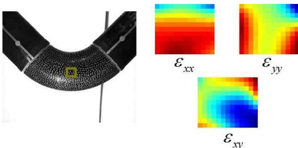
Fig. 1. Strain measurement using image signal
