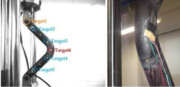
Fig. 3. Installed sensor (Targets and strain gage)
