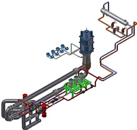
Fig.1 Graphic configuration of the RCP test facility
