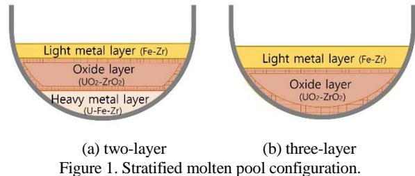
Figure 1. Stratified molten pool configuration.
