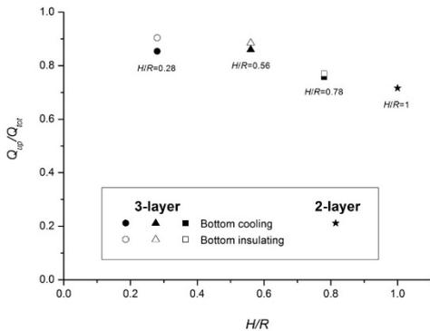
Figure 5. Upward heat ratio according to aspect ratios.
