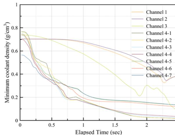
Fig. 7. Minimum coolant density
