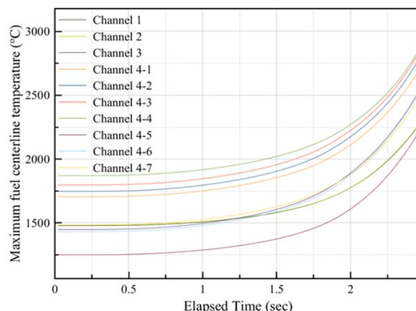
Fig. 5. Maximum fuel centerline temperature
