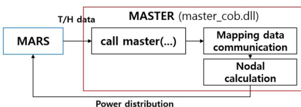
Fig. 1. MARS-MASTER coupling structure
