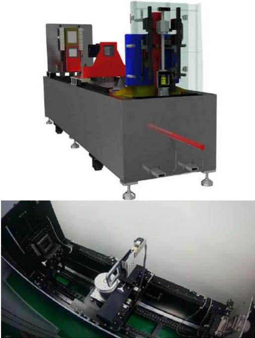
Fig. 4. (up) 3D drawing and (bottom) the prototype design of the high sensitive phase-contrast computed tomography system
