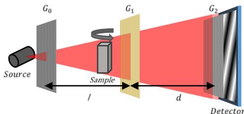
Fig. 1. Scheme of the Talbot-Lau grating interferometer
