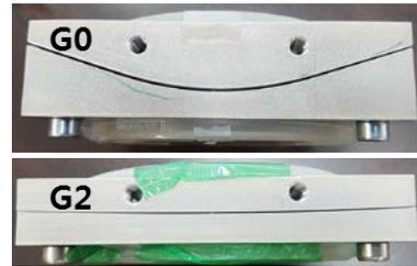
Fig. 3. Bending design to reduce shadow artifact
