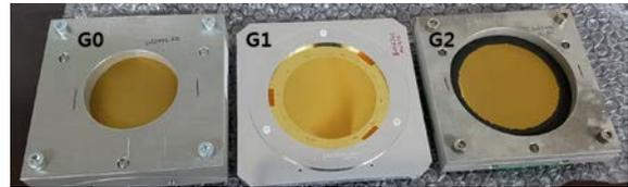
Fig. 2. Gratings for Talbot-Lau interferometer
