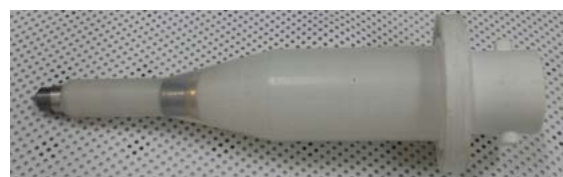
Figure 3. The miniature x-ray tube insulated by SR
