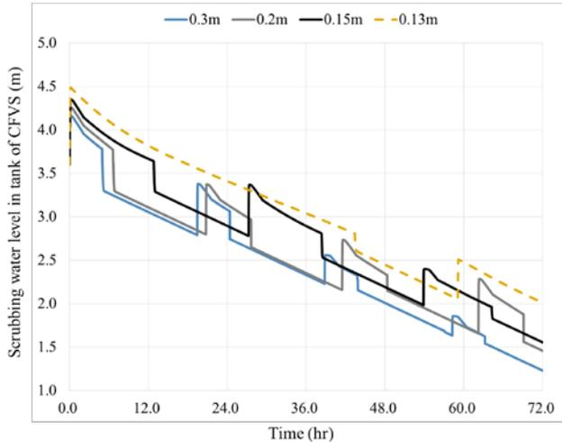
Fig. 5. Scrubbing water level in tank of CFVS
