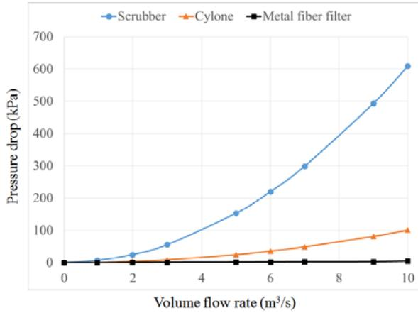
Fig. 2. Pressure drop of the scrubber, filter and cyclone
