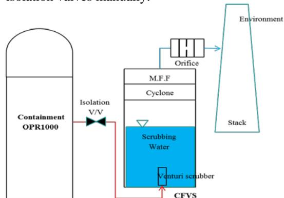
Fig. 1. Schematic of CFVS
