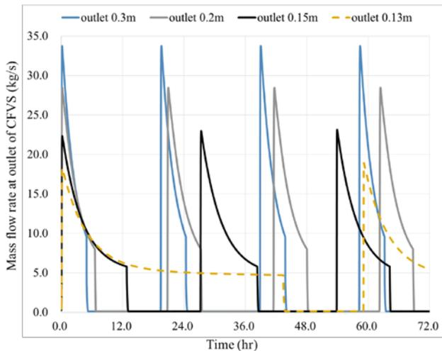
Fig. 6. Mass flow rate in CFVS (operating time: 72 hours)
