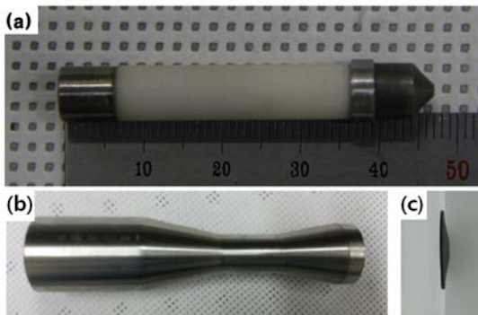
Figure 3. (a) An optical image of the fabricated X-ray tube. (b) X-ray shielding part and (c) X-ray flattening filter, respectively.
