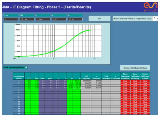
Figure 3. TTT diagram fitting for Ferrite/Pearlite phase of SA-516 Gr. 70 alloy.
