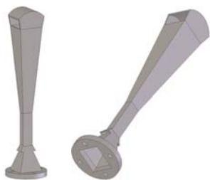
Fig. 1.1. Schematic of scrubbing nozzle
