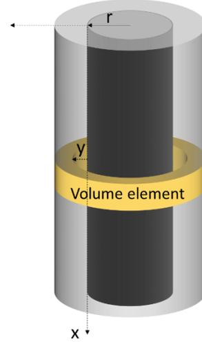
Fig. 5 Volume element of falling film along the string
