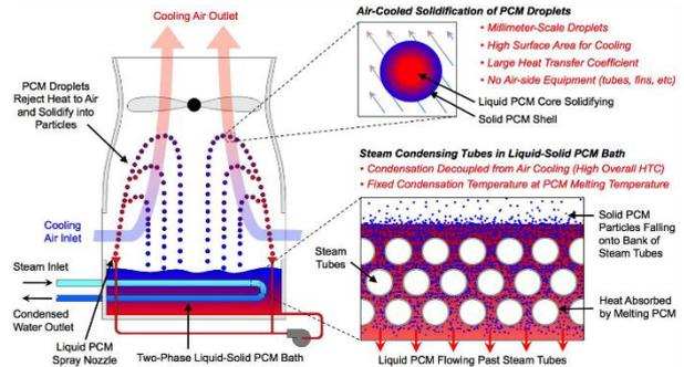
Fig. 2 Spray Freezing of Recirculating PCM (Drexel, USA)
