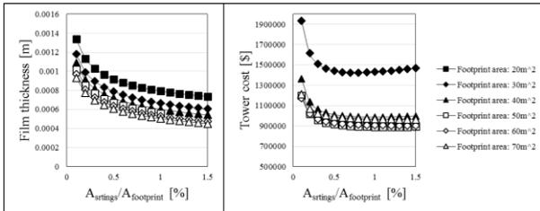
Fig. 8 Film thickness and cost analysis ( $r=1\text{ mm}$ )
