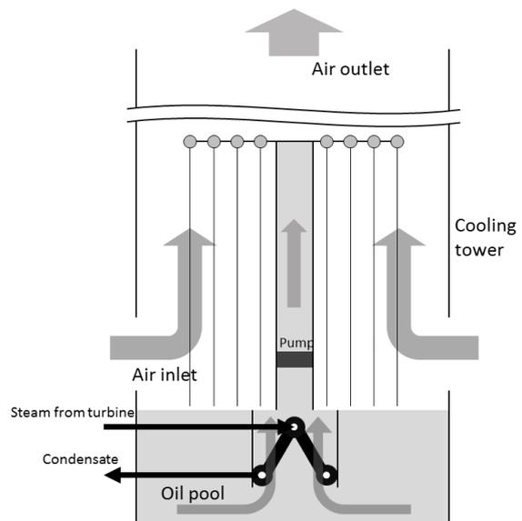
Fig. 3 Schematics of the dry cooled waste heat removal system
