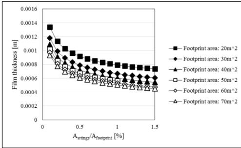
Fig. 7 Thickness of film along the strings ( $r=0.5\text{mm}$ )
