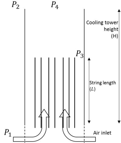
Fig. 6 Pressure points on the cooling tower
