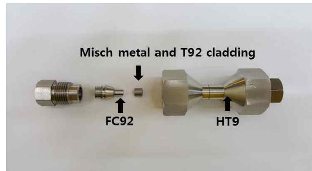
Fig. 1. Misch metal and jig for preliminary test
