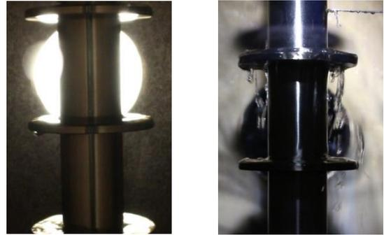
Fig. 3. Photos of the condensate on annular fins.
