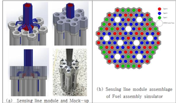
Fig. 4. Pressure sensing line extracting module.
