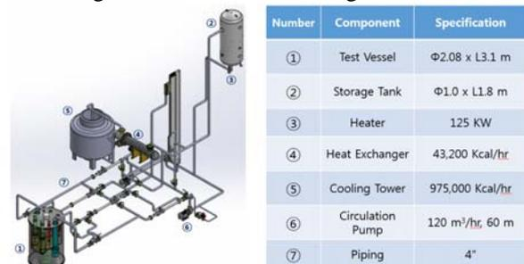
Fig. 1. Schematic of the Test Facility.
