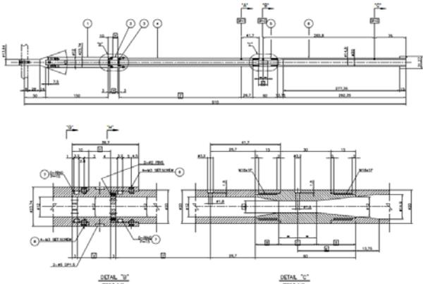
Fig. 3. Dimension of the fuel assembly simulator.
