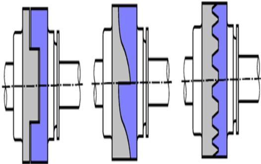
Fig. 1. Teeth type, claw clutch
