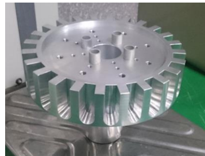
Fig. 2. Picture of the NTDHRD manufactured by aluminum.
