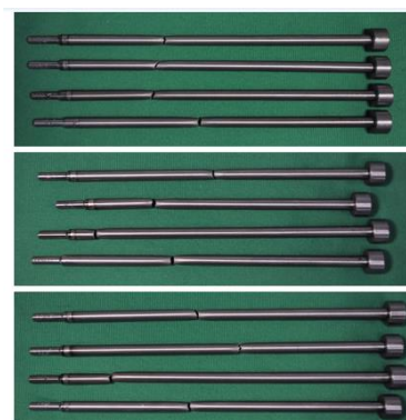
Fig. 7. Tensile test results (a)HT9, (b)FC92B, (c)FC92N
