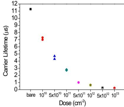
Fig.3 Change in carrier lifetime with irradiation dose
