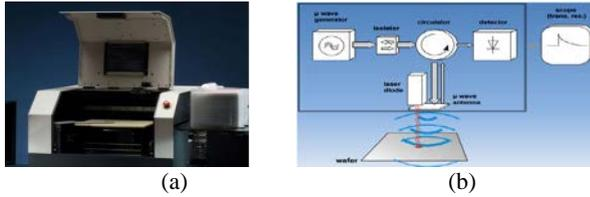
Fig. 2 (a) Semilab WT-2000, (b) The schematic of micro wave photoconductivity decay method
