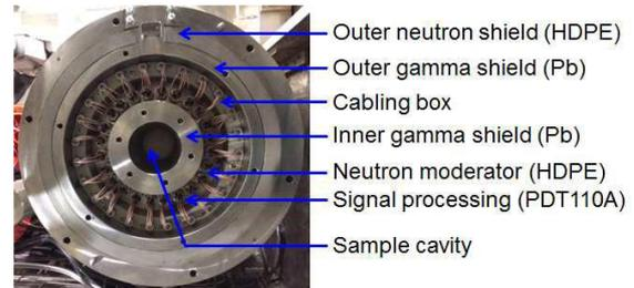
Fig. 1. Inner structure of fabricated ASNC.
