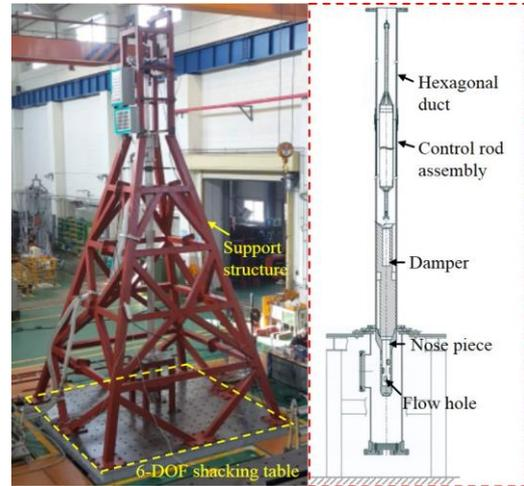
Fig. 1. Drop performance test facility.
