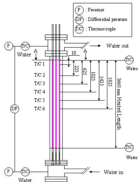
Figure 1. Schematic diagram for the test section.
