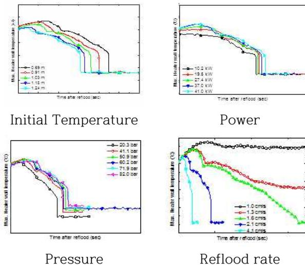
Figure 3. Influence of flow conditions on peak cladding temperature
