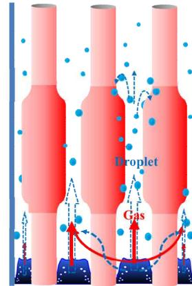
Figure 5 Flow distributions on the blockage region
