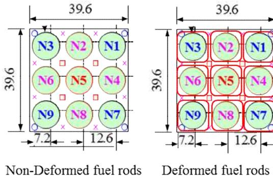
Figure 2. Geometry of 3x3 rod bundle
