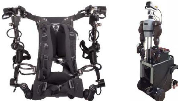
Fig. 1. The proposed system's exoskeletal master device and stair-climbing slave robot.
