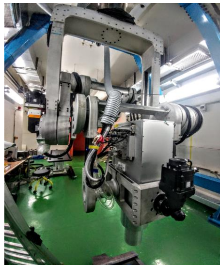
Fig. 2. 6 MeV LINAC mounted on a robot installed on the first floor at National Radiation Equipment Research and Fabrication Center
