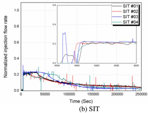
Fig. 2. Normalized injection flow rate
