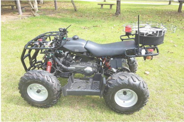
Fig. 1. Remote control system for accident monitoring (RAM)
