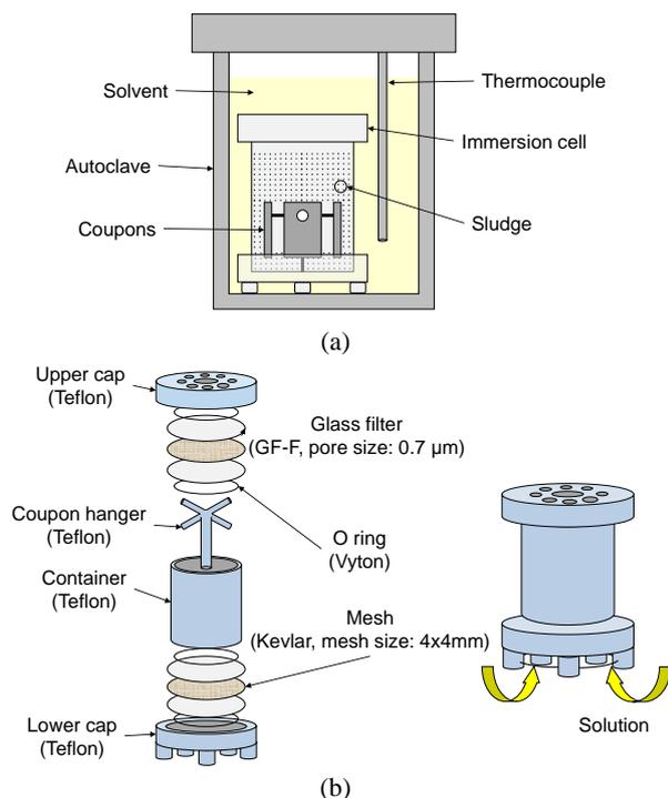
Fig. 1. Schematics of details of (a) autoclave and (b) immersion cell in chemical cleaning environments.
