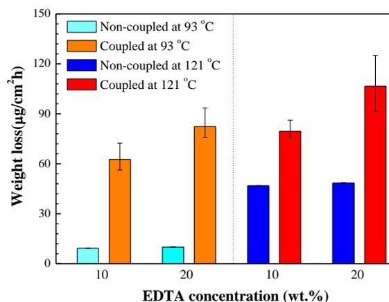
Fig. 2. Effects of magnetite, EDTA concentration, and temperature on the weight loss rate of SA508.
