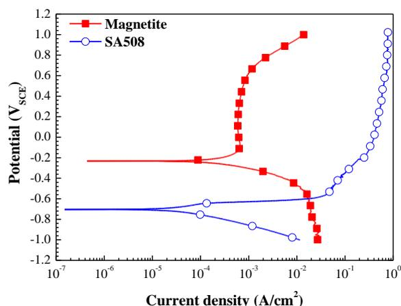
Fig. 5. Polarization curves of SA508 and magnetite in 10 % EDTA solution at 93 °C.
