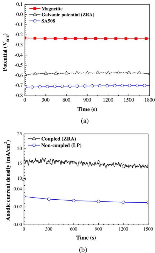
Fig. 6. Comparison of (a) corrosion potential and (b) anodic current density of SA508 coupled with and without magnetite in 10 % EDTA solution at 93 °C obtained by ZRA and LP technique.
