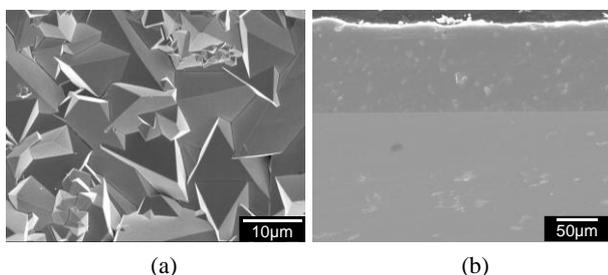
Fig. 4. SEM images of magnetite film electrodeposited on the SA508 substrate at the applied potential of  $-1.05 V_{SCE}$  in the deposition solution at 80 °C for 10 h: (a) top view and (b) cross section.
