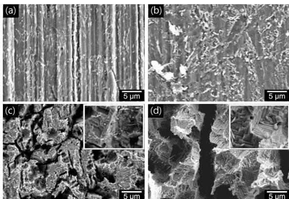
Fig. 3. SEM images showing the corrosion morphology of SA508 after immersion tests: non-coupled SA508 at (a) 93 °C in 10 % EDTA, (b) 121 °C in 20 % EDTA and coupled SA508 with magnetite at (c) 93 °C in 10 % EDTA, (d) 121 °C in 20 % EDTA.
